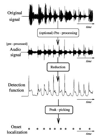
Fig. 2. Flowchart of a standard onset detection algorithm.
