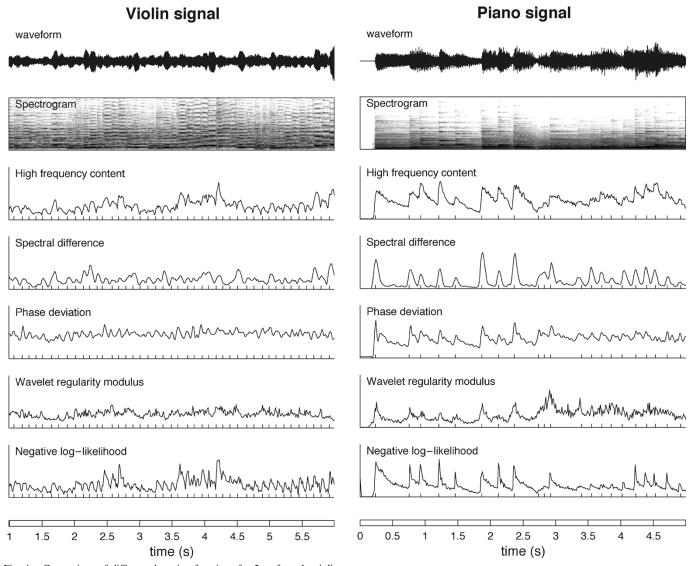
Fig. 4. Comparison of different detection functions for 5 s of a solo violin recording. From top to bottom: time-domain signal, spectrogram, high-frequency content, spectral difference, spread of the distribution of phase deviations, wavelet regularity modulus, and negative log-likelihood using an ICA model. All detection functions have been normalized to their maximum value.
